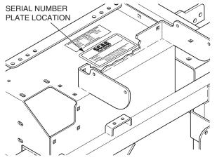
Figure 1-1. Mower Serial Number Plate Location
